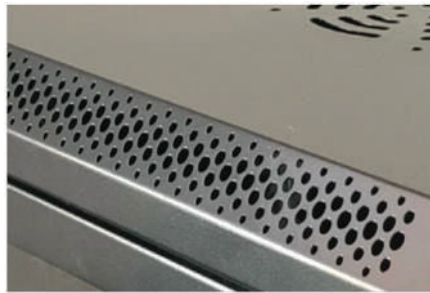
Front Ventilation Holes
