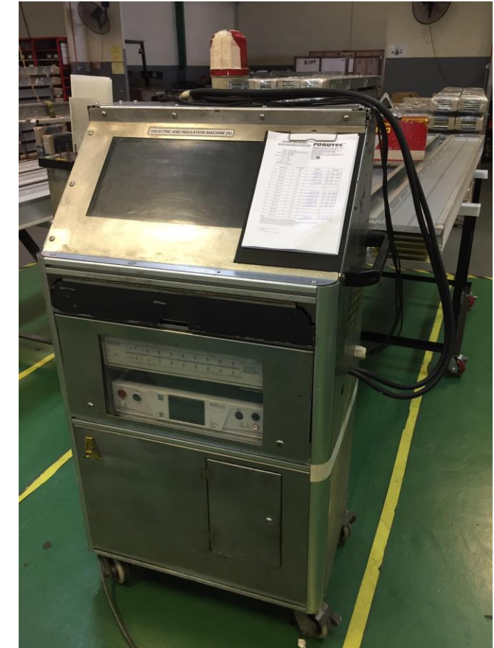
Dielectric Test (5kV for 5 Seconds and <100mA)
