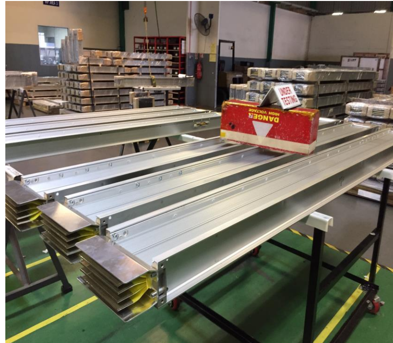
Insulation Resistance Test (DC1000V and >100MΩ)
